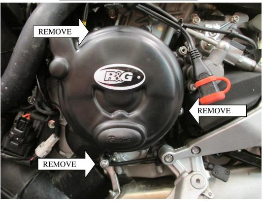
In this kit there should be: 1x Engine Case Cover (ECC0194R) 3x M6 x 35mm long Cap Head Bolt 1 x Racing Puck (SK0001SK (already fitted)) 2 x PAL Nuts (already fitted)
