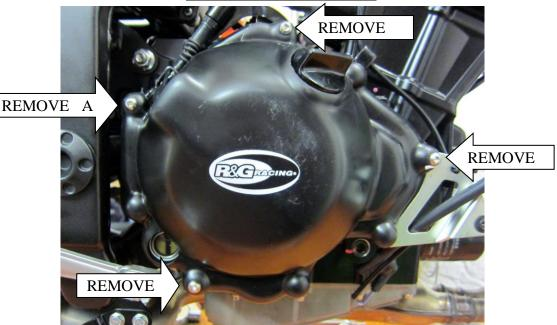
In this kit there should be: 1 x Engine Case Cover (ECC0140) 3 x M6x40mm CAP HEAD BOLTS 1 x M6x35mm CAP HEAD BOLTS
